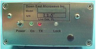
IF transceiver of 10 watts or less and a 10 GHz antenna system. The 10368-144LP model (low power) is a basic design that can be used as a portable rig or integrate into an existing system. It's output level is perfect for most TWT amplifiers or to use for short mountain top contacts. The gain and noise figure of the 144LP is reciprocal for it's TX power level, but adding a high performance LNA and a power amplifier makes it a top notch system.
