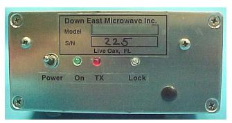
The DEM 10368-144 or 10368-144LP is a complete transverter ready to go transverter needing only an IF transceiver of 10 watts or less and a 10 GHz antenna system. The 10368-144LP model (low power) is a basic design that can be used as a portable rig or integrate into an existing system. It's output level is perfect for most TWT amplifiers or to use for short mountain top contacts. The gain and noise figure of the 144LP is reciprocal for it's TX power level, but adding a high
