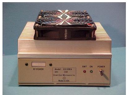
This amplifier design utilizes the combining of four Mitsubishi RA18H1213G MOSFET hybrid power modules. All regulated voltages and biasing that are required for proper operation are self-contained.
