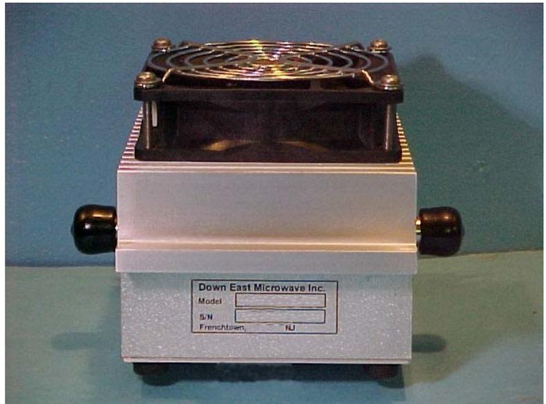
This amplifier design utilizes the Mitsubishi RA18H1213G MOSFET hybrid power module. All regulated voltages and biasing that are required for proper operation are self-contained.
