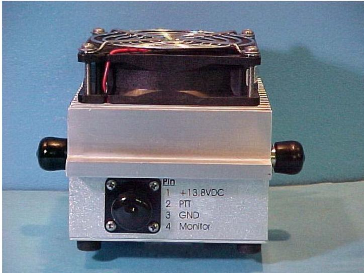
Use high quality coaxial cables on both RF connections. At 1300 MHz., VSWR and insertion loss become factors even in the shortest lengths of coax. Test all coaxial components at low levels before installing into the final system.
