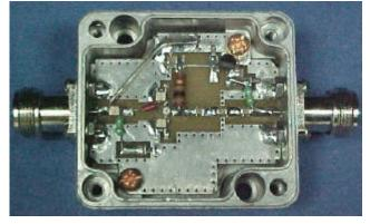
Down East Microwave Inc.'s LNAWPQ low noise amplifier design incorporates a shunt L, series L input circuit and a resistive loaded output circuit. During the test process, the input circuit is optimized for gain, noise figure and attenuation below 500 MHz. The resistive loaded output circuit, is adjusted to control the gain and is tested for a constant wide band-width output impedance. This resistive load impedance absorbs products caused by reflections from band
