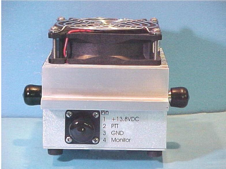
Install the amplifier with the heat sink on top or with the fins vertical so the amplifier will convection-cool. A variable speed fan is supplied to pull air through the heat sink fins and will cool the amplifier in any mode of operation including continuous duty applications. It is recommended not to keep the amplifier continuously keyed in the transmit mode without applying RF drive.
