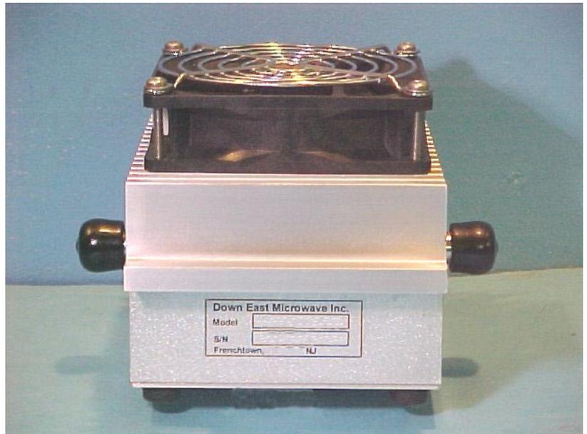
The RF power monitor supplies a relative DC voltage to RF power.
