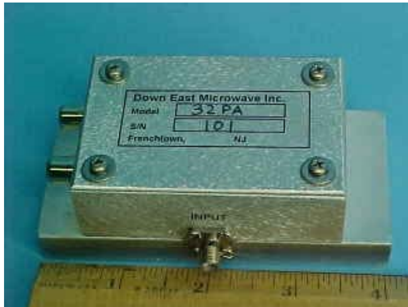
3-3PAP needs to be mounted to existing Box or heatsink
