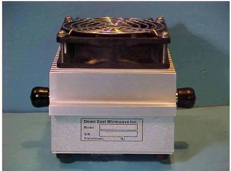
This amplifier design utilizes the Mitsubishi RA20H8994M MOSFET hybrid power module. All regulated voltages and biasing that are required for proper operation are self-contained.
