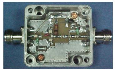
Down East Microwave Inc.'s LNAWPQ low noise amplifier design incorporates a shunt L, series L input circuit and a resistive loaded output circuit. During the test process, the input circuit is optimized for gain, noise figure and attenuation below 500 MHz. The resistive loaded output circuit, is adjusted to control the gain and is tested for a constant wide band-width output impedance. resistive load impedance absorbs products
