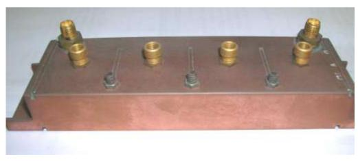
The filters measure 5.8" long (including mounting flange) by 1.5" wide. Total height will depend on the length of tuning screw utilized but top of the SMA connector is under 1.25". If purchased un-tuned, this document will provide the basic procedure to produce a 5760 MHz filter.
