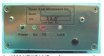
The DEM 5760-144 or 5760-144LP is a complete ready to go transverter needing only an IF transceiver of 10 watts or less and a 5.7 GHz antenna system. The 5760-144LP model (low power) is a basic design that can be used as a portable rig or integrate into an existing system. It's output level is perfect for most TWT amplifiers or to use for short mountain top contacts.
