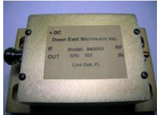
Mechanically, the converter is housed in a weather proof aluminum housing that is chemical treated to prevent oxidation. It is provided with mounting brackets to be attached to any mast or mechanical structure that your antenna is mounted to.
