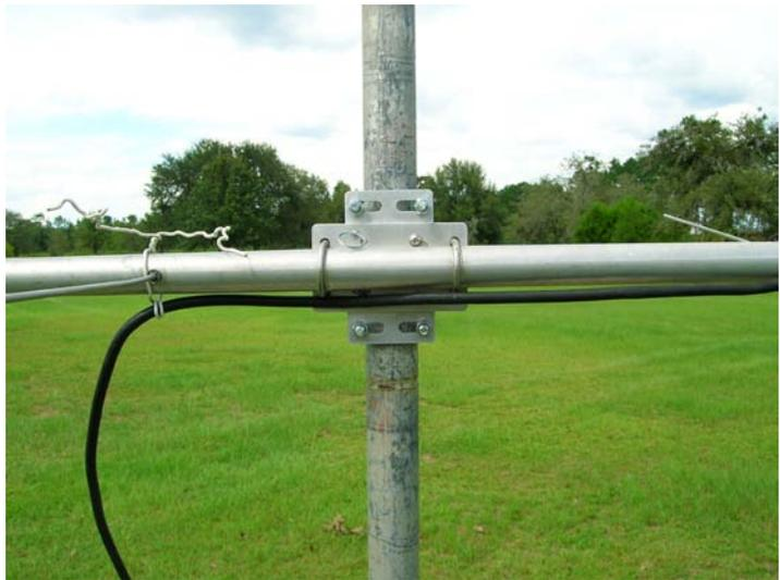
The QDAM is designed to fit up to 1-1/2" boom diameter antennas utilizing 1/4" U-Bolts for attaching to the BOOM plate. The BOOM plate will accommodate 1/4" U-Bolt sizes of 1" inside to a 2" outside measurement. Depending on the antennas boom size, the U-Bolts should be selected to provide best fit. The MAST plate may be mounted to a maximum of a 2" mast
