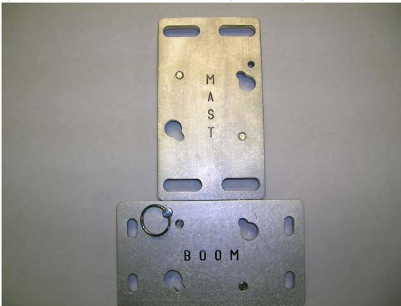
with 5/16" U-Bolts. The MAST plate, with its larger slots as pictured to the left, can utilize a 5/16" U-bolt size of less than 1" inside to a 2.7" outside measurement. If mounting the MAST plate to a larger mast diameter up to 2.20" is required, utilizing a 1/4" U-Bolt will accomplish it. Then because of the flatness of the plate, all square booms and masts may be used up to the maximum U-Bolt size that fits.
