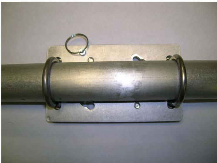
Next, mount the BOOM plate to the antenna. The word “BOOM” should face the antenna boom. As mentioned before, the boom-to-mast plate that is being replaced should have the required 1/4” hardware but don’t hesitate to replace anything worn or galled. Again, saddles may be utilized but standard lock and flat washers will work perfectly. Be sure to center the U-Bolts of they are undersized for the slots.
