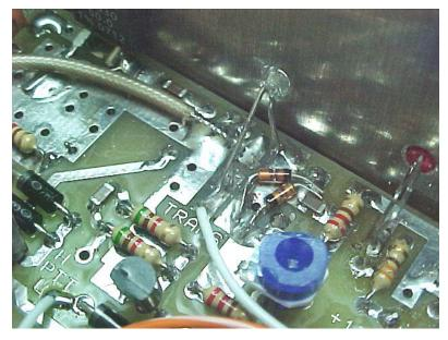
when you are utilizing the internal source of the DigiLO, the transverter ON LED will be lit. When you connect the external 10 MHz source, the LOC LED will light and the ON LED will shut off. Consider the transverter on and active if either LED is lit.
