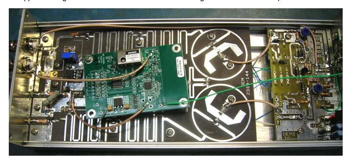
Use two 4-40 x 1/2" standoffs and lock washers to replace the existing 4-40 screws and directly bolt the board in place or use ground lugs and solder them to the board holes after alignment. Then use the replaced screws to hold the board in place. Be sure to orientate the board as shown. The example is the 2304 transverter on the previous page and 3456 below. BUT-- there are other hole combinations that will work for both transverters.
