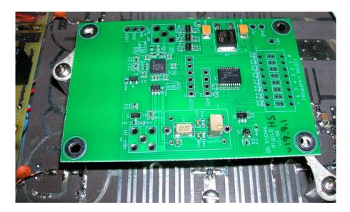
Attach the coax from the transverter to the RF OUT of the DigiLO and the wire to the +V. Make them as short as possible. Install a BNC connector in the rear panel for the external 10MHz input(if you desire to use one) and connect a coax from the connector to the REF IN on the DigiLO as shown in the 2304 picture.
