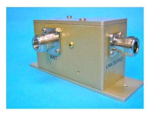
Secondary mounting holes are tapped for  $4-40 \times 5/16$ " and are spaced 1.50". They are located on the ANT side of the relay.
