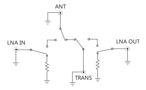
Schematic shows relay in TX position, DC removed. All 4 relays fire at once during RX.
