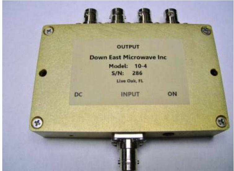
**OPERATION:** The assembled DEM L10-4 is easy to use. There are no adjustments to make or levels to set. Just simply connect a DC supply between 11 and 18 VDC that can source 200 mA. Then connect your 10 MHz input signal not exceeding +10dBm. The 4 outputs will then produce the same level output (+/- 1 dB) of 10 MHz signal with the harmonic level being less than -35dBc.
