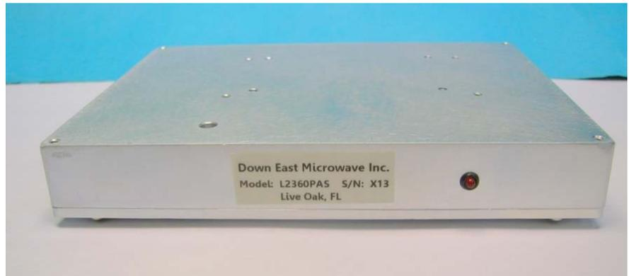
damage may occur. If this option is ordered there will be an additional Installation document provided and will contain a template to aid attachment to any type of conduction cooling device. There are 8 attachment holes within the L2360 enclosure and are tapped to 4-40 size. Further clearing or adjustment may be required to ensure that the amplifier enclosure fits flush with the assembly it is attached to.
