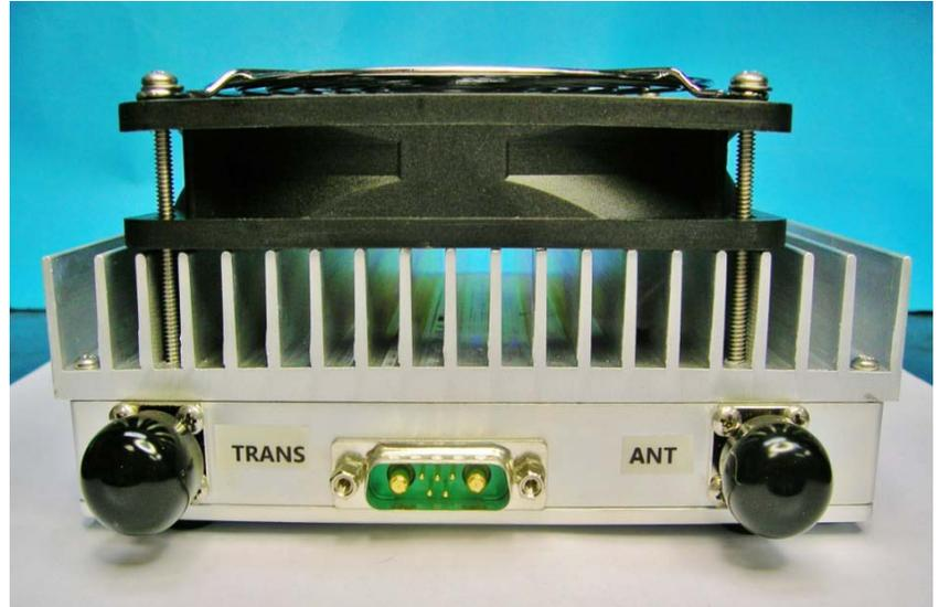
**Power Output and Input Drive Levels:** The Linear output power is optimized for a minimum level for the required input drive level. Head room is allowed to enable full linearity of the amplifier and a higher compressed output power. If FM mode operation is the only requirement, the amplifier will be optimized for a compressed output power.
