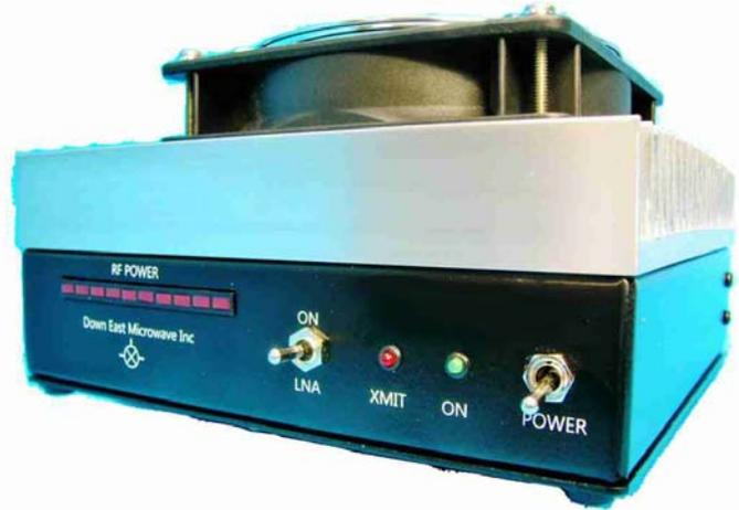
Plus, it offers the ability to change the IF frequency range (28 or 144 MHz) at any time. The new design also includes other improvements over past versions by offering a 4 step sequencer, bypass control of an external mast mount LNA if desired, and remote DC power control. All of this with a standard 25 watt output power level.
