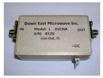
a slight degradation in specifications at the band edges while meeting or exceeding the specifications above somewhere in the band. The LNA is assembled in a machined chemical etched enclosure with SMA connectors only. It is biased through an external DC feed through connector. The LNA will withstand input RF levels of up to 20 mW.
