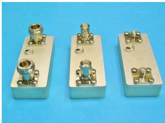
For frequency specific LNA's, low loss filters on the input and/or output circuits are implemented to develop the standard or custom frequency LNA's. All frequency specific LNA's are delivered with optimized gain and noise figures.
