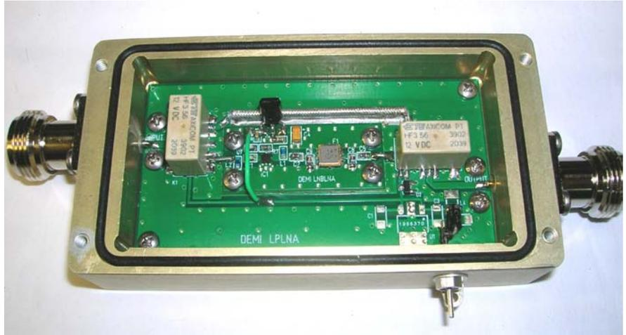
feed thru connection to allow connecting to your sequenced system for transceivers that do not have their own LNA control function. It is an ideal LNA for any type of weak signal work including satellite operation utilizing any standard transceiver power level in the VHF/UHF region.
