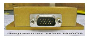
supplied) of up to +30 VDC. All DC input and output connections are made through a DB-15 connector and has one Dual function LED. Transmit or Receive.
