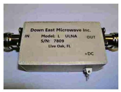
Our LXXULNA design incorporates low loss microstrip circuitry and resistive loading to accomplish all RF matching. During testing, the input circuit is optimized for gain and noise figure.
