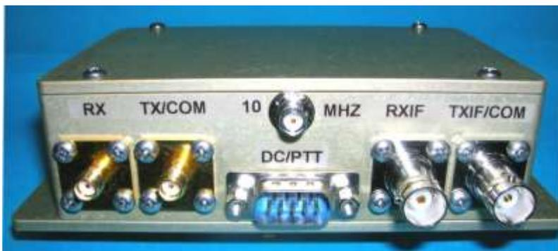
The MINI2304 will be provided with a wired DC/PTT cable and be ready to use after completing the simple set-up procedure. Because of its small size (4.5" x 3.0" x 1.5") a flanged cover plate is included with a provision to attach it to any fixed surface. The cover plates may be interchanged if it allows for easier
