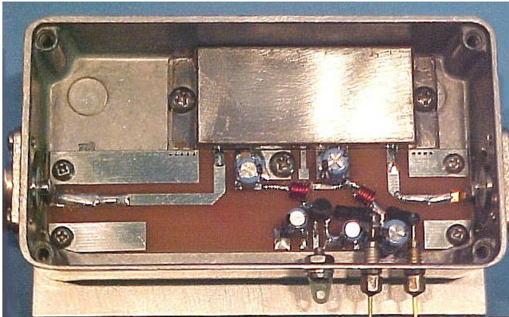
In combination, the screw holds the bottom of the PCB down to the heat sink to ensure the shortest path of the by-pass capacitors to modified flange of the hybrid. The addition of the shield after it is soldered to the ground connections on the PCB is to now reduce the inductance even further. This design is now unconditionally stable and ready for the RF test.
