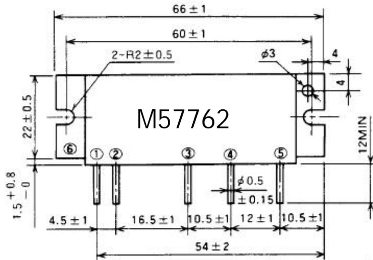
**Figure 2. Physical dimensions of modules.**
