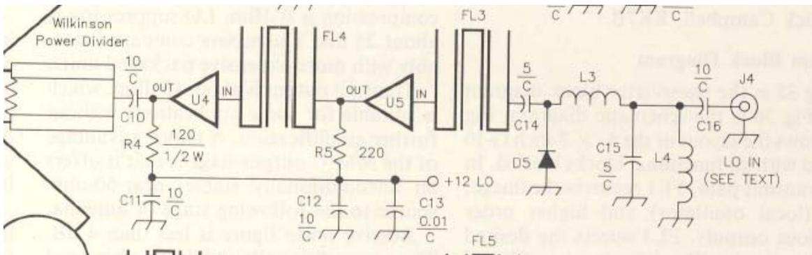
It is a two-mixer design with a Wilkinson power divider. The mixers requires +7dBm, therefore, the divider requires +10dBm. This can be accomplished by modifying the attenuator pad value on the A-32 and directly injecting the signal into the power
