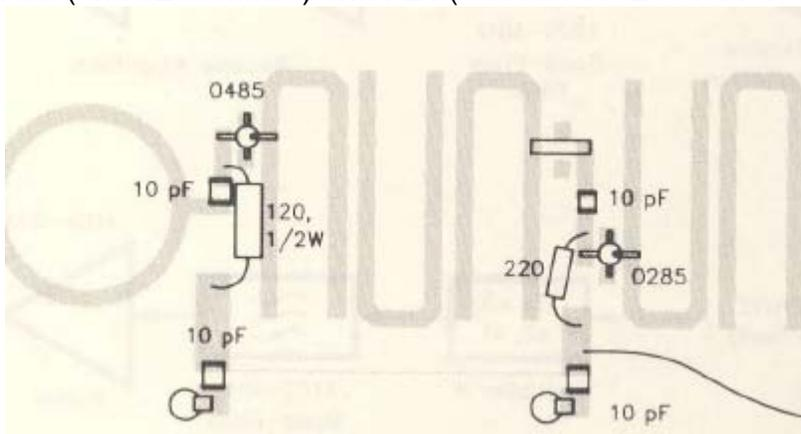
utilized for the input from the A-32 at any frequency around 1152 MHz. No attenuation changes are required on the A-32. The 220 ohm bias resistor to U5 is removed of course along with the original SHF LO and then replaced with the A-32 circuit.
