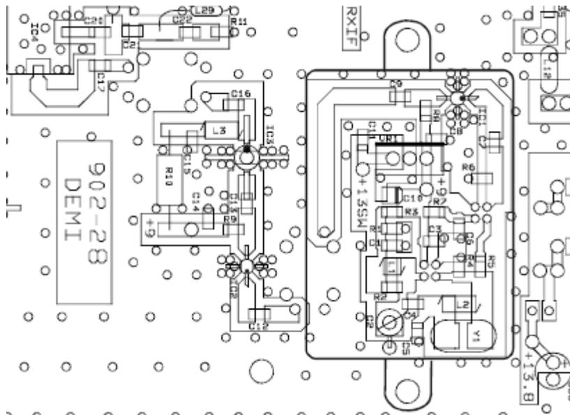
would encounter is the model change for the 3 and 10 watt transverters using Hybrid power modules to the newest model utilizing 1 watt MMIC's. During this design transition, the 9-volt regulator was moved from the oscillator shield area to outside on the board bolted to the enclosure. The two different component placements are shown for clarification. The regulator is required to supply DC power to the MMIC's in the LO chain. To disable the
