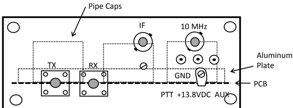
Attach all of the 8-32 feed thru connectors and the required **BNC connectors**. If you desire a common IF, receive and transmit through a single connector, only install one BNC. If you desire separate Receive and Transmit IF connections, install both BNC connectors. Be sure to install the lock washer and the ground lug on all **BNC connectors**.
