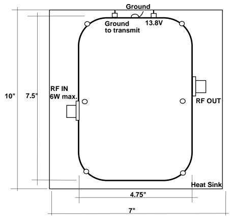
Note: The heat sink option model is 12" L x 10" W
