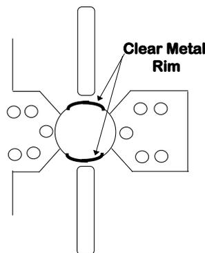
**Figure 1. MMIC PC Board hole with metal rim**
