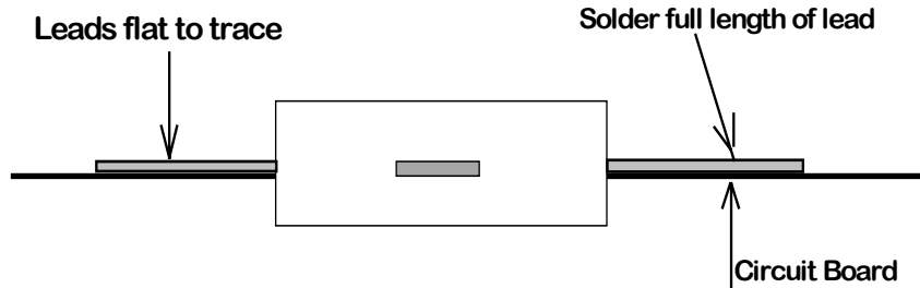
Figure 3. U1-U5 MMIC Installation (Also see addendum)
