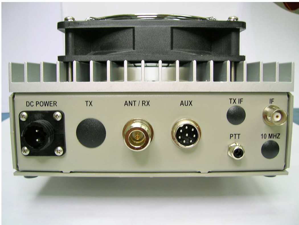
34. Rear view of transverter and fan install.
