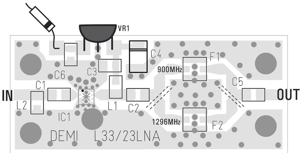
After the correct filter is selected by disabling the other, install the 78L05 regulator VR1, and C4 as shown above. Cut the leads of the regulator to 3/8" or less and attach to the circuit board. Then be sure to observe the polarity of C4 before installing. The banded end is the Positive. Then install the Diode as shown above.
