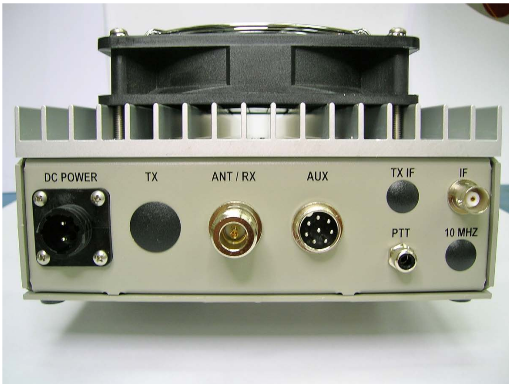
33. Rear view of transverter and fan install.
