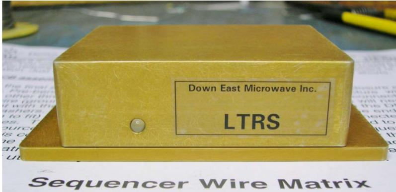
Our new DEM LTRS Sequencer is a copy of the solid state sequencer we have utilized in our past VHF/UHF and Microwave transverter designs. It is similar to our previous design by WB5LUA but without the relays, making it a completely solid state unit. As in previous designs, this sequencer is intended to be used with any lash-up that requires separate sequenced switching circuits to control pre-amps,
