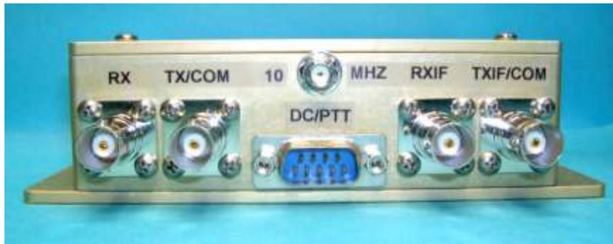
Apply power to the system and verify that it is in receive mode. The Lock LED should be lit on the MINI and will be RED if you are utilizing its internal source or Green if you are using a external 10 MHz source. Next verify the receive noise floor. With all of the system equipment on, the MINI's RXIF gain can be adjusted to a comfortable
