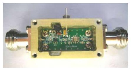
Band Pass filters. The LNA's do not offer any RF bypass switching for transceiver operation and therefore may only be utilized in receive only applications. It is offered with a robust machined enclosure and various types of RF connectors and connector combinations. Overall enclosure size without connectors is 1.75" L x 1.0" W x 0.9" H
