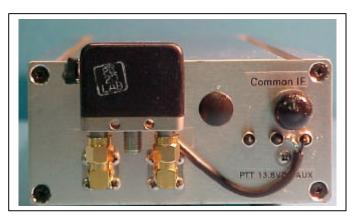
The Down East Microwave10 GHz. assembled transverters are available as model number DEM 10368-144 (2 watt version) and 10368-144LP (low power version). Complete kits are available as the 10368-144CK and the 10368-144LPCK. The PC board kit is only available as a low power transverter, the 10368-144K. PC boards only are available for the low power transverter as the 10368-144PCB. The 10368-WTR may be ordered with a kit or assembled unit. If ordering the WTR option,
