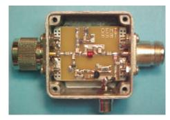
watt transmission for up to one minute. It is switched in the transmit path when it senses a accidental transmission. The SSBT is housed in a 2" x 2" x 1.2" die cast enclosure with 2 RF and 1 DC connectors.
