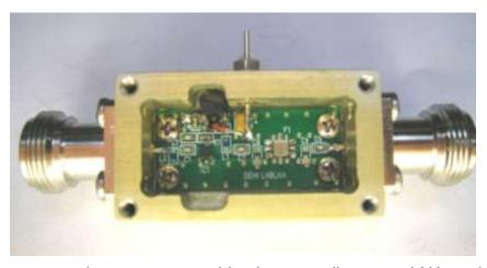
and various types of RF connectors and connector combinations to allow any LNA to be "dropped in" to any pre-existing system or is ready to be component in a newly developed receive system. A bias through the coax option is available.
