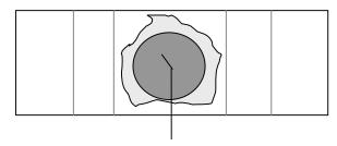
3. Shape the brass into a clamp by bending it away from the Thermistor to simulate the figure below. Do not bend the tabs excessively. One shot would be best! Many re-shapings will cause the brass to fatigue and break off.
