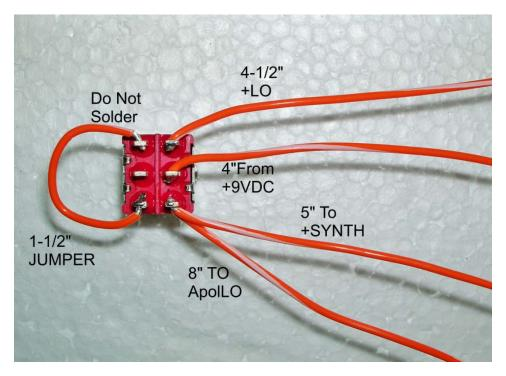
After completion, install the switch in the enclosure so that the +9VDC side of the switch (right hand side of the picture) is closest to the side wall of the transverter. The open center terminal of the switch connects to the +13.8 VDC wire from the transverter. The unsoldered wire connection gets doubled up with the +13.8SW wire on the transverter board. Wire and solder both of those connections now.
