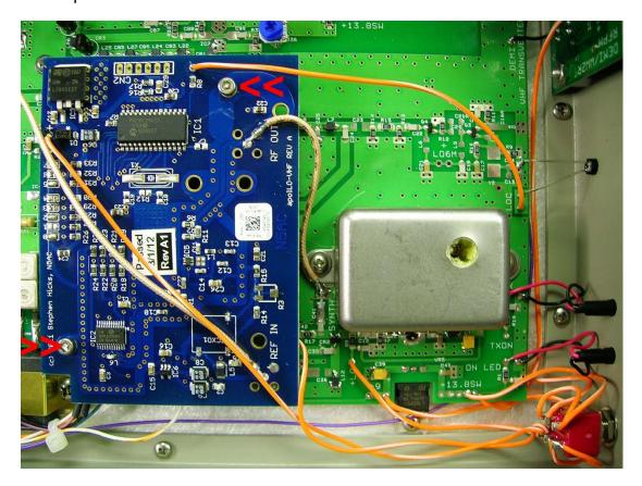
Finish the wiring by attaching the 8-1/2" coax end to the REF IN, the 3" coax to the RF OUT and the 8" wire to the + all on the VHF ApolLO board. If you do not desire the dual oscillator option, install a 8-1/2" wire from the + on the ApolLO to the top side solder tab on the power switch. Finish all versions by connecting a 4-1/2" wire from the LOC pad on the transverter board to the via near R8 on the ApolLO.
