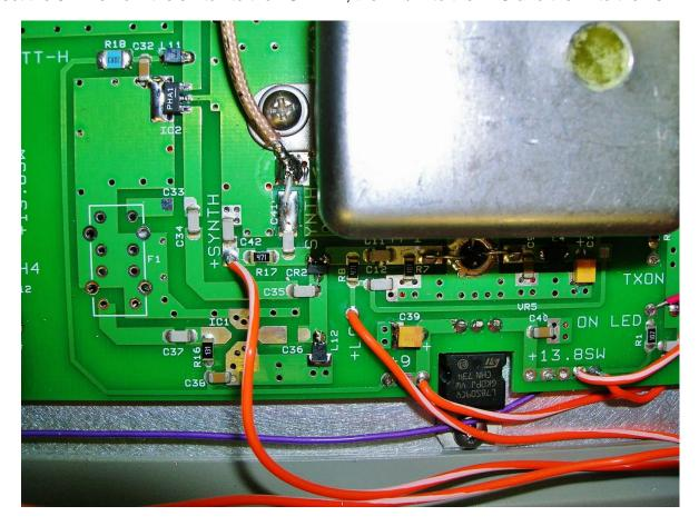
If you are only utilizing the ApolLO and not the standard oscillator, install a 2" jumper between the +SYNTH and the +9 connections.
