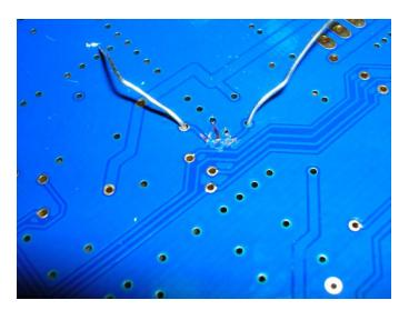
solder mask by scraping it with a sharp knife to ease the soldering of the transistor
