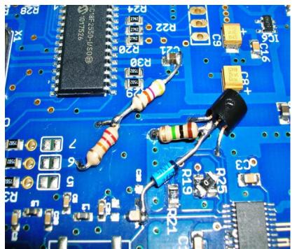
Next, attach the 22K, 47 K and 1 Meg resistors as shown. If the via holes are covered with solder mask, scrape them clean before component insertion. Make short lead connections as shown.
