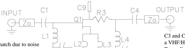
Any mismatch due to noise matching C1/L1 improves input IP3
